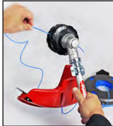
2. Feed the trimmer line through the head
