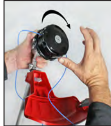
4. Twist head "clockwise" until ~8" trimmer line shows
